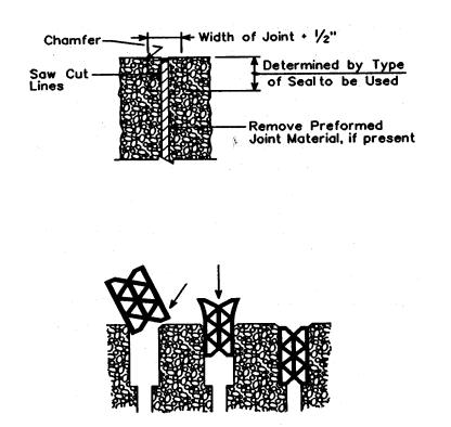
Exhibit X.27 Upgrading Joint to Accommodate Compression Seal
