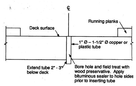
Exhibit X. 9 Drain tube to remove water trapped between planks.
