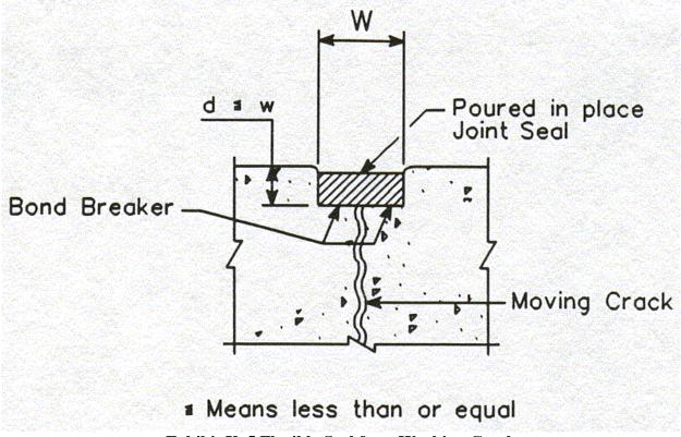
Exhibit X. 5 Flexible Seal for a Working Crack
