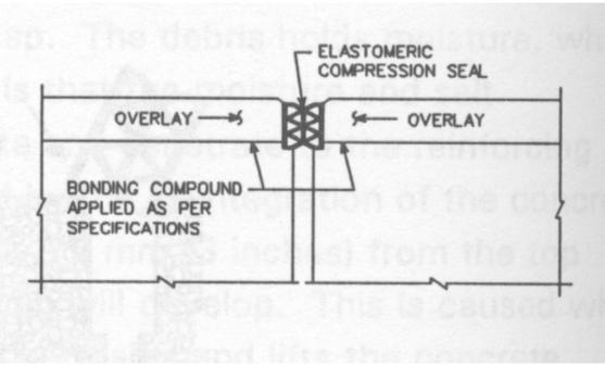
Exhibit X. 28 Installation of compression seal with overlay
