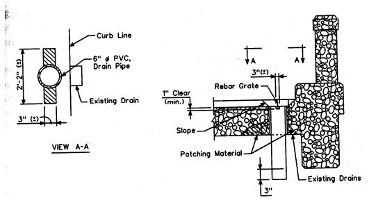
Exhibit X.34 PVC Deck Drain Installation
